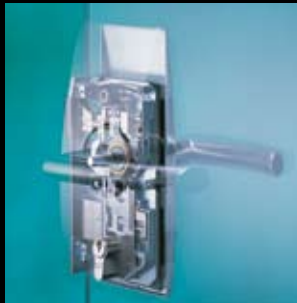
DORMA ARCOS Office Lock. Lock case with its exception- ally rugged functional com- ponents designed to satisfy the requirements of the type approval test performed to DIN 18251, Class 3.
